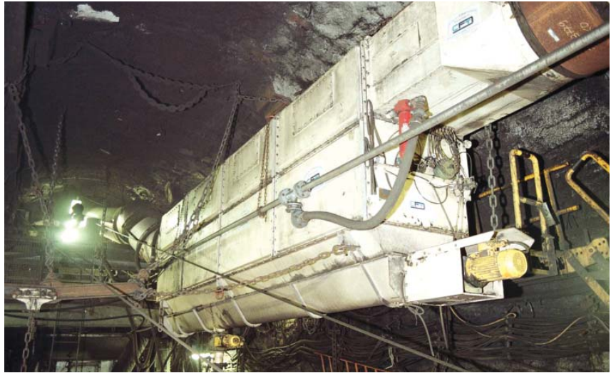
A CFT dry deduster for underground mining. (Photo: CFT)
